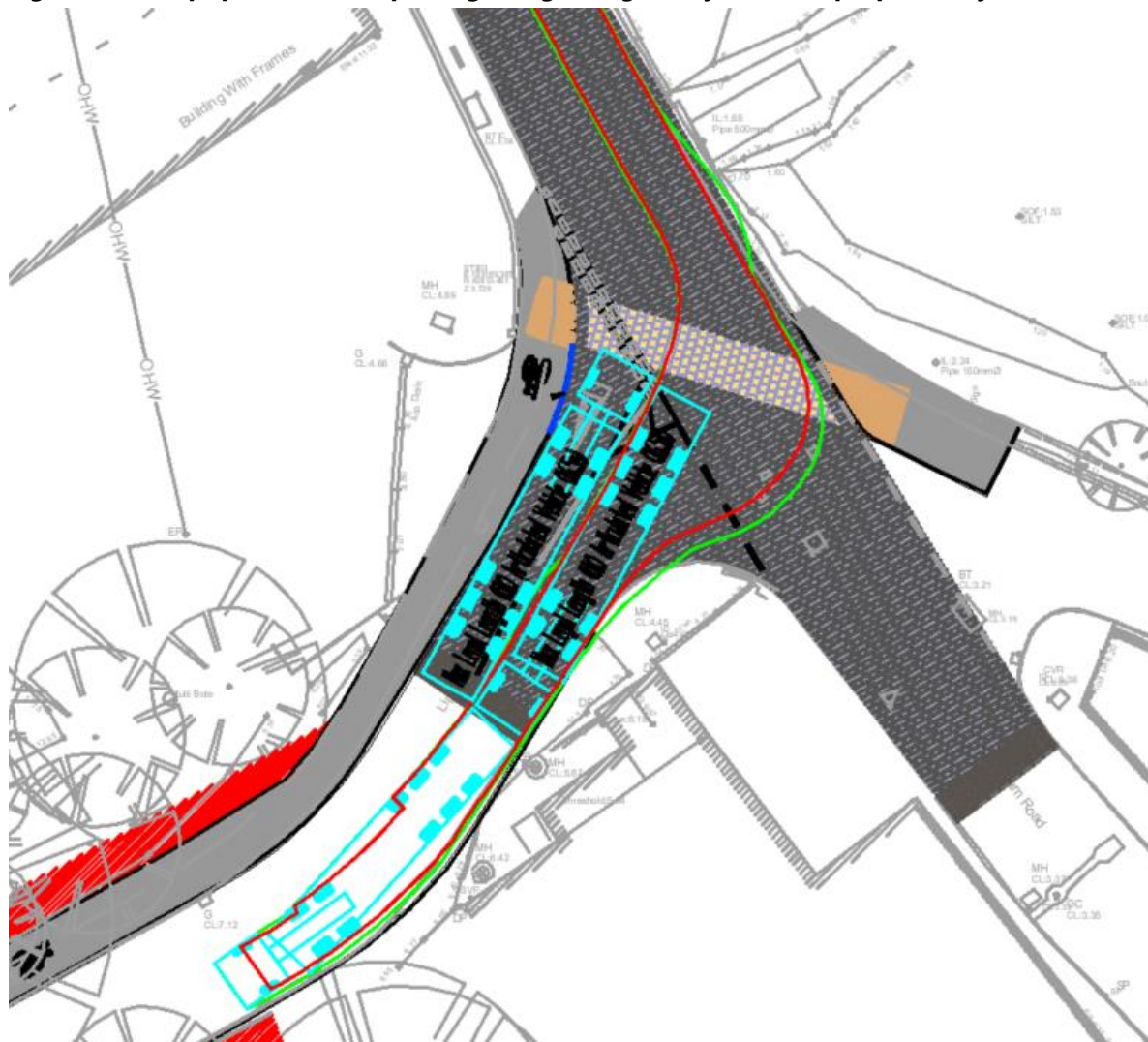
Figure 2 - Swept path of HGVs passing at Lighterage Hill junction – proposed layout
